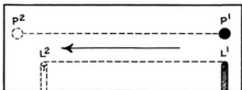
B.-TRAVEL OF SHADOWS WHEN PALPATOR IS RAISED HIGHER THAN PROJECTILE TUBE BEING SHIFTED IN CONTRARY DIRECTION
