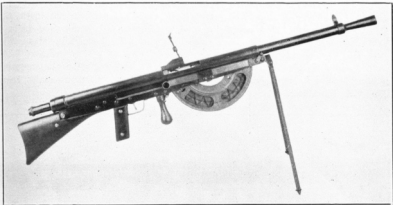
FIG. 52.—Chauchat machine rifle, model 1915, caliber 8 mm.
