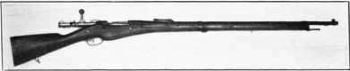
FIG. 44—French Lebel rifle, model 1907-15. In this model a clip-loading magazine under the receiver was substituted for the cylinder magazine of the 1886-93 model; otherwise the gun was practically the same as the latter. The magazine holds three cartridges loaded in a clip
