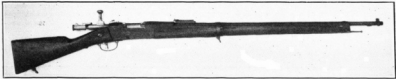
FIG. 43.—French Lebel rifle, model 1886-93. This rifle, the standard arm of the French Army at the beginning of the war, had a tubular magazine under the barrel.
