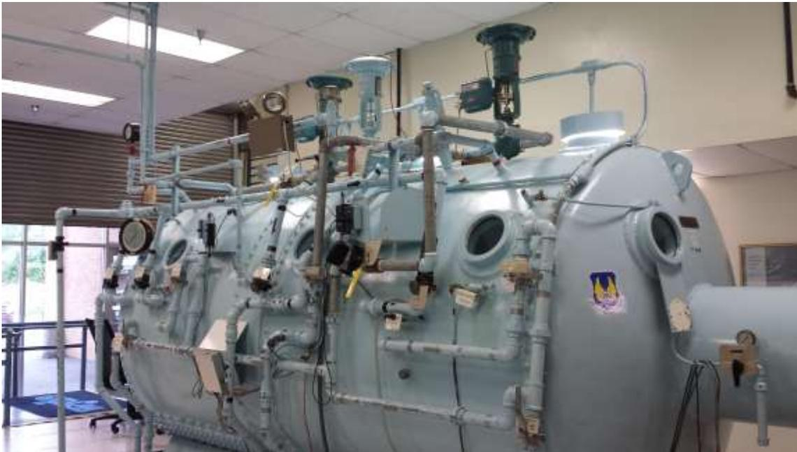
The caisson today, at Brooks City Base. The rivets were kept for the historical look, but the joints were welded in the 1964 renovation. The caisson can be visited at Brooks City Base.
